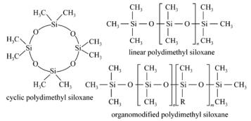
Figure 6 Structures of polydimethyl siloxanes and their derivatives
