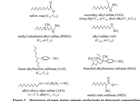
Figure 1 Structures of some major anionic surfactants in detergent compositions
