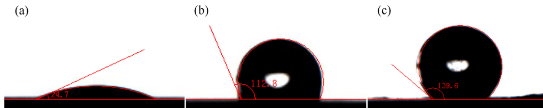
Fig. 1. Contact angle of GCC particles (a) unmodified; (b) after aqueous mixing with RCOONa; (c) with thermal treatment (220 °C, 60 min) after aqueous mixing.
